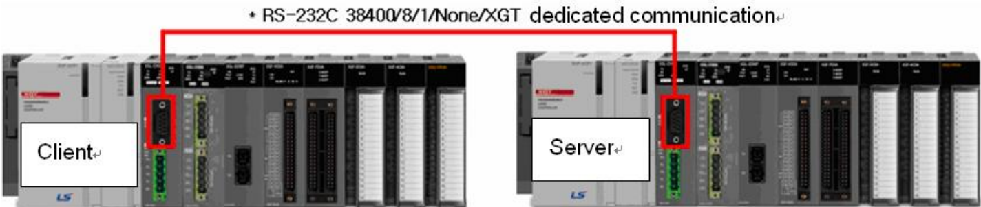
[Figure 10.1] example of dedicated system configuration
