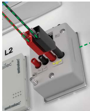
Ex: Voltage sensors measurement
